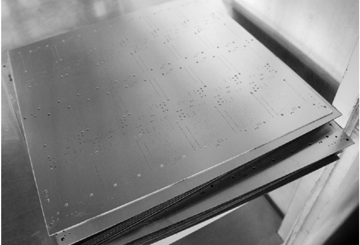
A stack of finished, drilled panels of Arduino Leonardo boards
