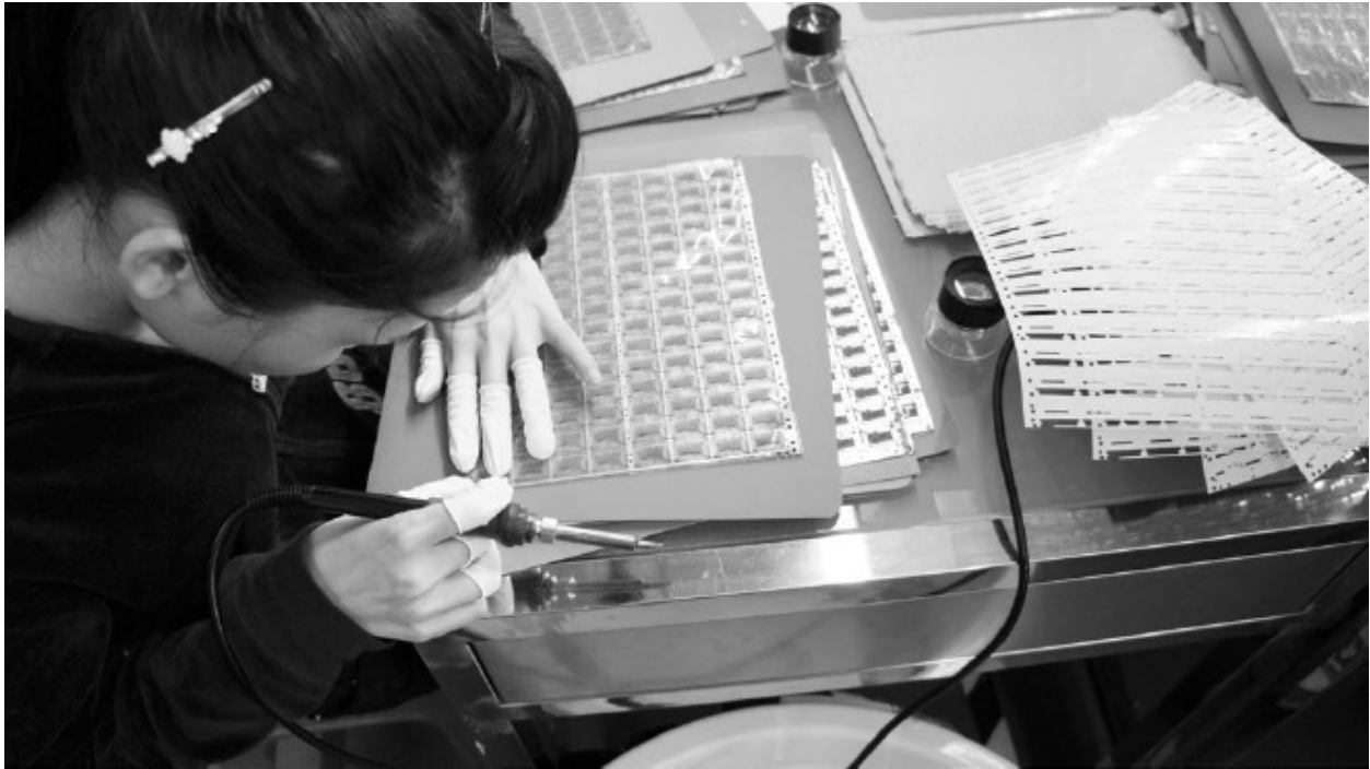
A worker manually aligning coverlay onto flex-circuit material
