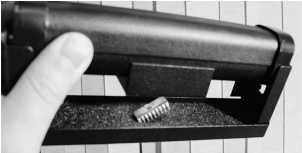
The chip in the UV eraser's antistatic foam
