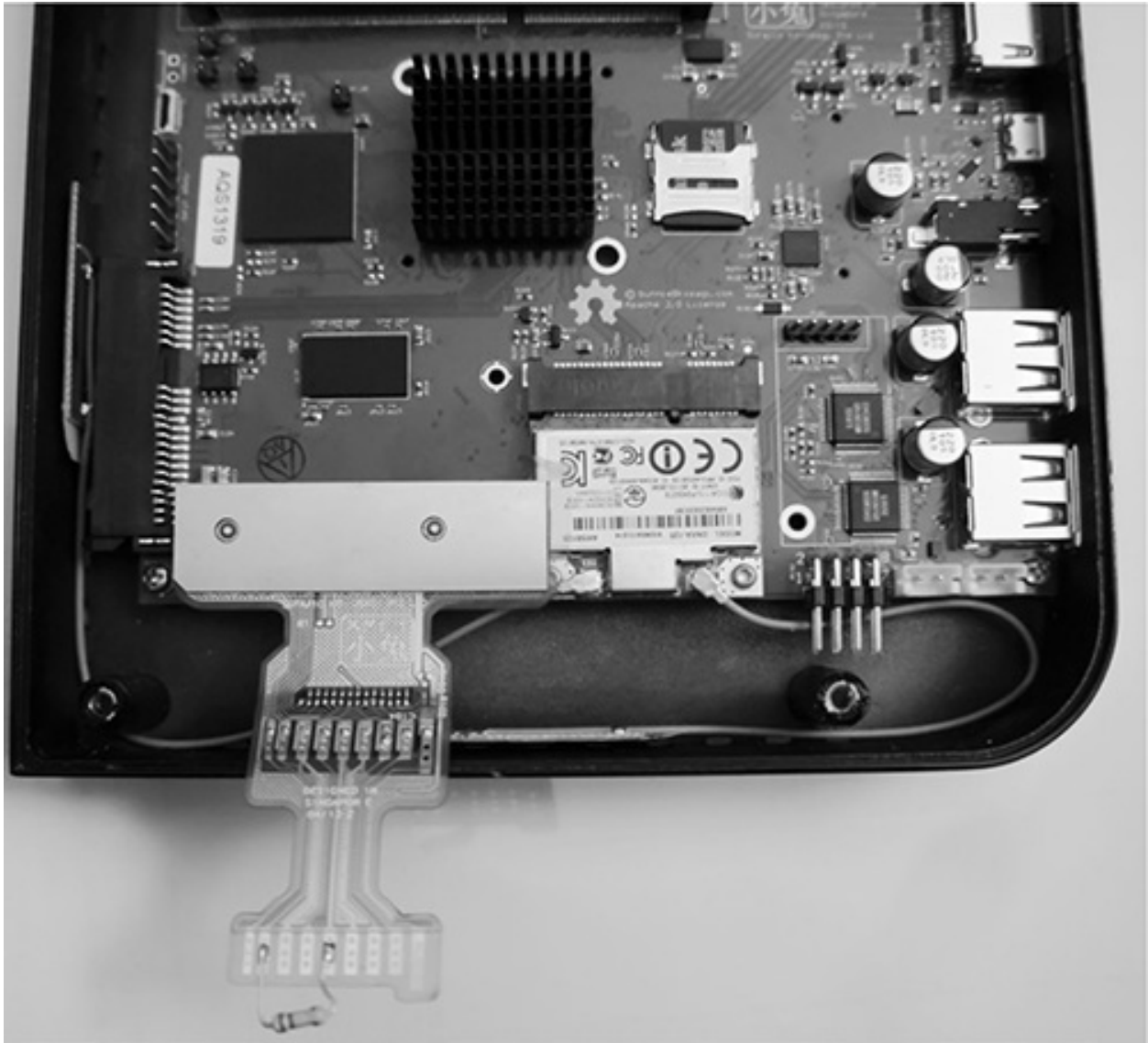
A flex-circuit adapter plugged into a Novena
