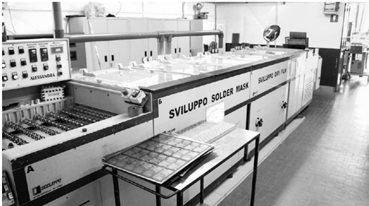
The machine that develops the photoresist
