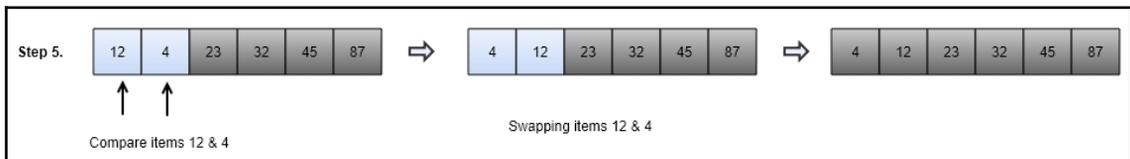
The implementation of the bubble sort algorithm would work in a double-nested loop, where the inner loop repeatedly compares and swaps the adjacent elements in each iteration for a given list, and the outer loop keeps track of how many times the inner loop should be repeated. The implementation of the inner loop is as follows:
