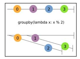
We can further understand how <code>group\_by</code> works with a simple example. Let's say that we want to group the number according to the fact that they're even or odd. We can implement this using <code>group\_by</code> by passing the <code>lambda x: x % 2</code> expression as a key function, which will return 0 if the number is even and 1 if the number is odd:
