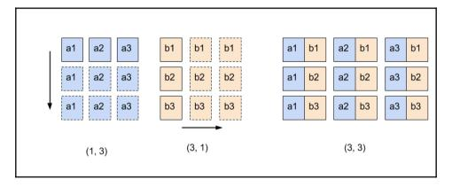
Using code, our strategy will be to transform the a array from shape (3,) to shape (3, 1), and the b array from shape (3,) to shape (1, 3). The two arrays are broadcasted in the two dimensions and get multiplied together using the following code:
