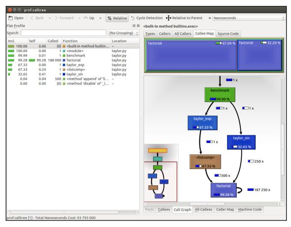
The preceding screenshot shows the KCachegrind user interface. On the left, we have an output fairly similar to <code>cProfile</code>. The actual column names are slightly different: **Incl.** translates to <code>cProfile</code> module's <code>cumtime</code> and **Self** translates to <code>tottime</code>. The values are given in percentages by clicking on the **Relative** button on the menu bar. By clicking on the column headers, you can sort them by the corresponding property.
