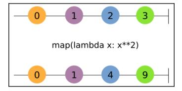
The source observable is placed at the top of the diagram, the transformation is placed in the middle, and the resulting observable is placed at the bottom.
