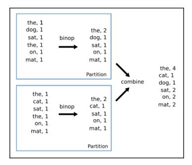
The following code illustrates how to use Bag and the foldby operator to compute the word count. For the foldby operator, we need to define two functions that take five arguments:
