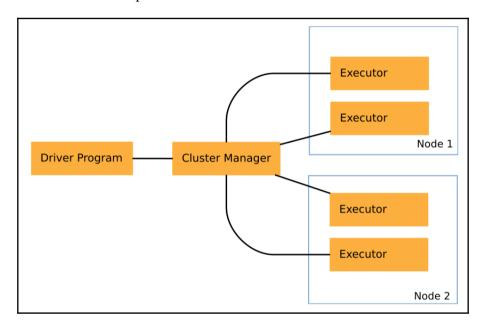
A natural question to ask is: How is Spark, a software written in Scala, able to execute Python code? The integration is done through the Py4J library, which maintains a Python process under-the-hood and communicates with it through sockets (a form of interprocess communication). In order to run the tasks, Executors maintain a series of Python processes so that they are able to process Python code in parallel.
