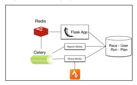
A typical deployment will group the Flask app with one Redis and one Celery instance on the same server and serve requests through a web server such as Apache or nginx. The database can be located on the same server, or on a dedicated server.
