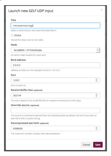
Once the new input is in place, Graylog will bind the UDP port 12201 and will be ready to receive data. The docker-compose.yml file has that port exposed for the Graylog image, so your Flask applications can send data via the localhost.
