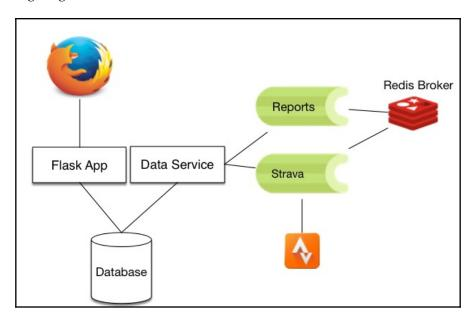
The Data Service is an HTTP API that wraps the database containing all the users and runs data. The dashboard is the frontend that implements the HTML user interface.
