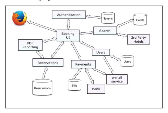
Don't be afraid of the number of components displayed in this diagram. The internal interactions of the monolithic application are just being made visible by separate pieces. We've shifted some of the complexity and ended up with these seven standalone components:
