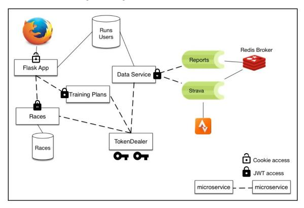
JWT access in this diagram means that the service requires a JWT token. Those services may validate the token by calling the TokenDealer. The Flask app in this diagram needs to obtain tokens from the TokenDealer on behalf of its users (link not shown in the diagram).
