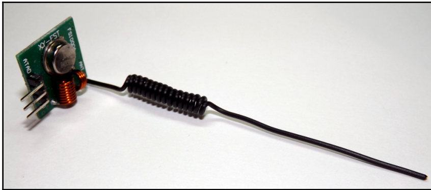
The transmitter range is vastly improved with a simple antenna
