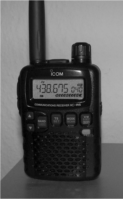
Figure 8.15 The Icom IC-R5 is a reliable tool for capturing a variety of common frequencies.
