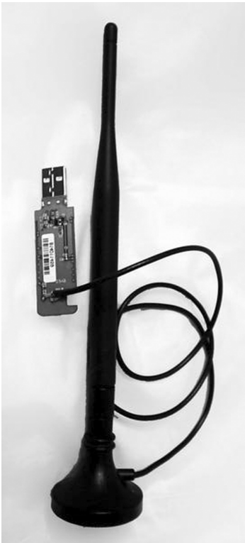
Figure 8.7 Bluetooth adapter with hacked connector and antenna.
