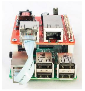
Figure 6-9: A Raspberry Pi with a PoE HAT (hardware added on top).
