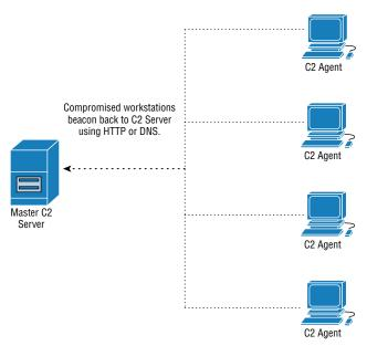
Figure 8-1: Initial beacon designated as Master node.
