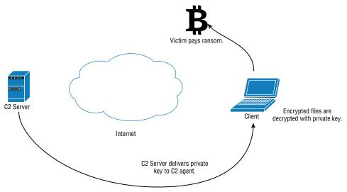
Figure 5-4: Decryption process flow.
