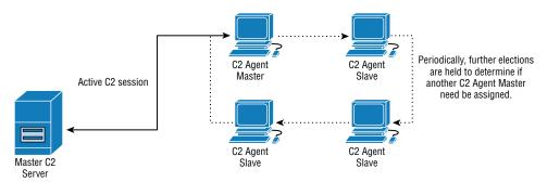
Figure 8-7: Further elections are held as necessary.
