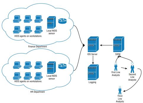
**Figure 3-2:** A basic intrusion monitoring setup.
