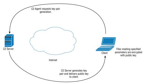
Figure 5-3: Encryption process flow.
