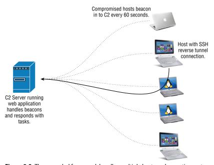
Figure 2-3: The upgraded framework handles multiple hosts and operating systems.
