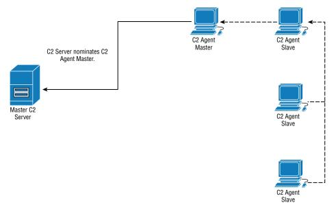
Figure 8-2: C2 uses Master for outbound connectivity.
