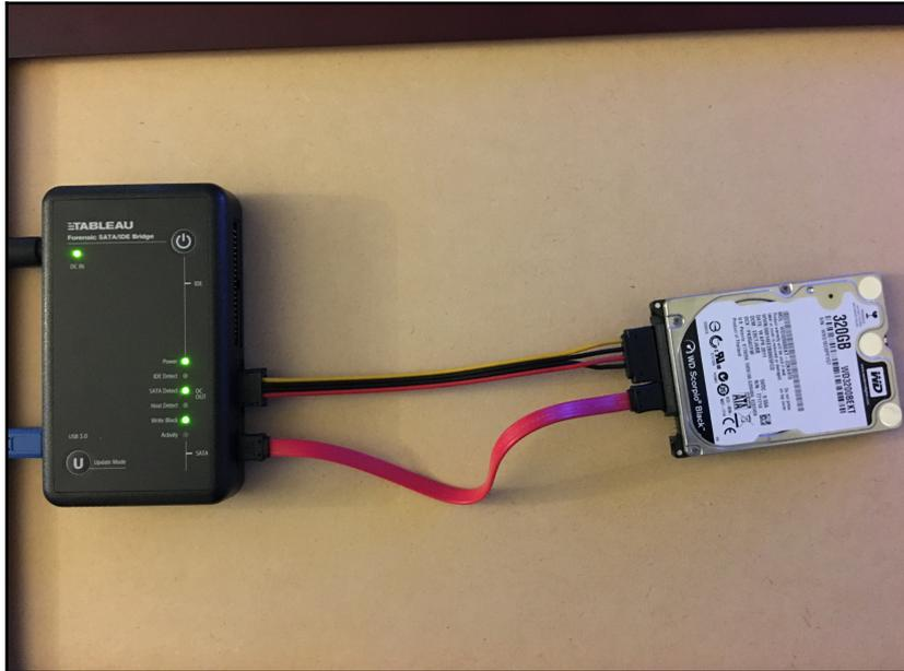
6. With the physical write blocker in place, the suspect drive is now ready for imaging. In this example, the freeware application FTK Imager will be used. FTK Imager requires administrator privileges to run. Open the executable and the following screen will appear:
